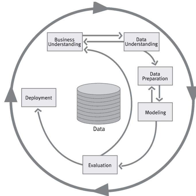
Figure 3.2: CRISP-DM Process Model
