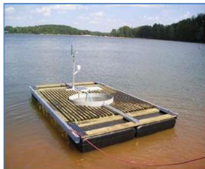
Figure I.5. Bac flottant (Stan et al., 2016).
