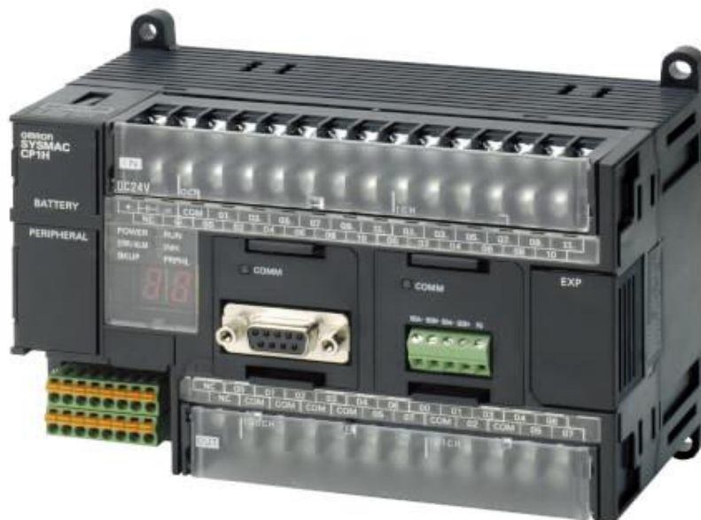
Figure 20: Automate programmable Industriel
