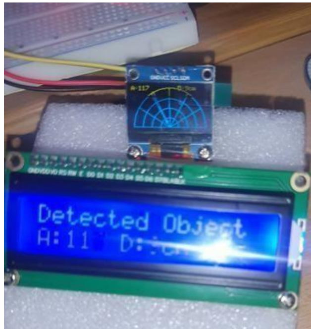
Figure III.4: Displayed angular scanning of the ultrasonic sensor.
