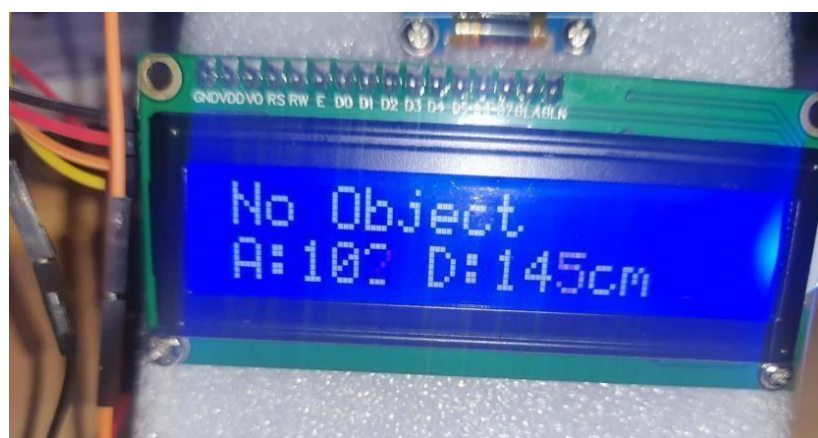
Figure III.5: Distance measurement using the ultrasonic sensor.
