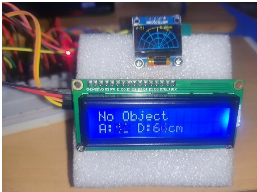
Figure III.6: LCD and SSD1306 OLED module displaying real-time information.
