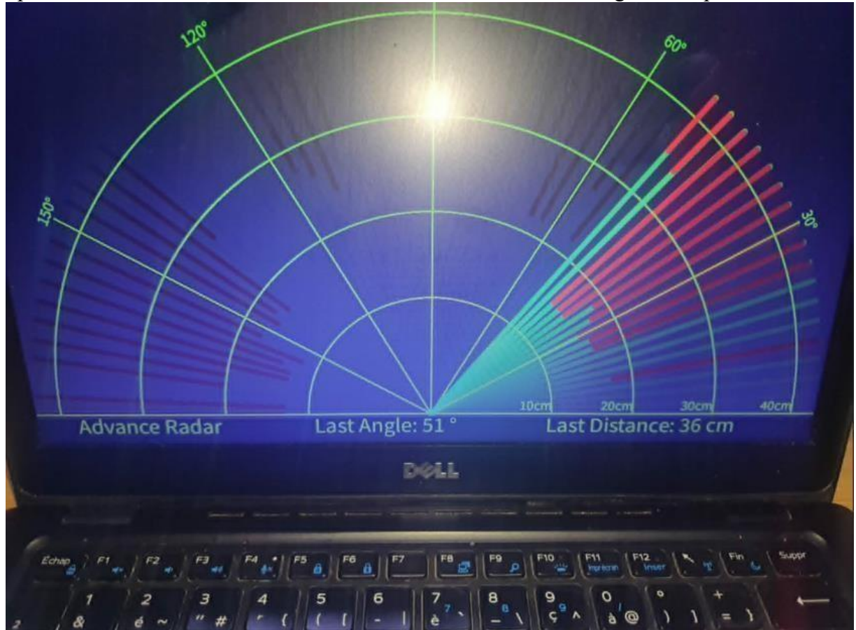
Figure III.8: Processing interface for ultrasonic radar visualization.
