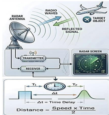
Figure I.1: Reflection of the transmitted wave from a target.
