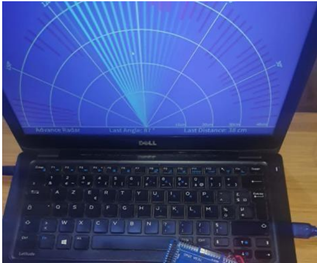
Figure III.7: COM port communication with Processing interface.
