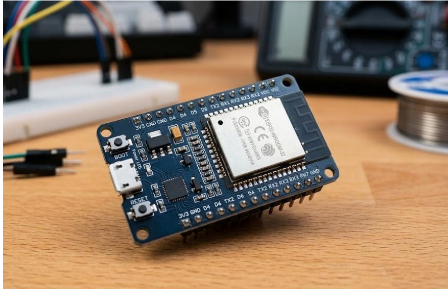
Figure III.5 : ESP32 Microcontroller used as an Edge Computing Node
