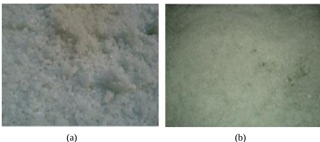
Figure II.15 : (a) fritte opaque, (b) fritte transparente
