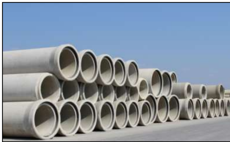
Fig. V.01. Conducts of concrete armed.
