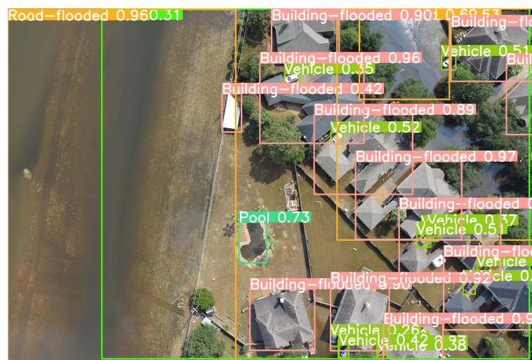
Figure 3.9: Examples 01 of visual results for the Object Detection using YOLOv8
