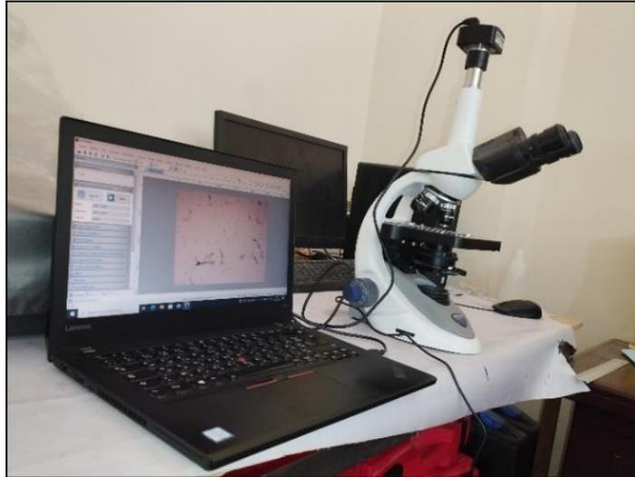
**Figure 53 :** Microscope OPTIKA (trinoculaire optika C-B3A). [\(photo original\)](#).
