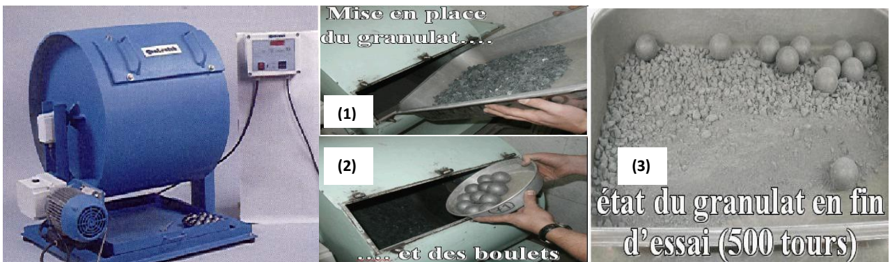
Figure. II.13. essais Los Angeles
