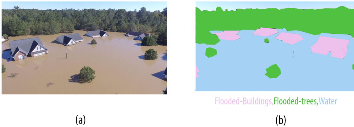
Figure 1.6: Sementic segmentation of flooded aerial,(a)Image Original,(b)Image Segmentation
