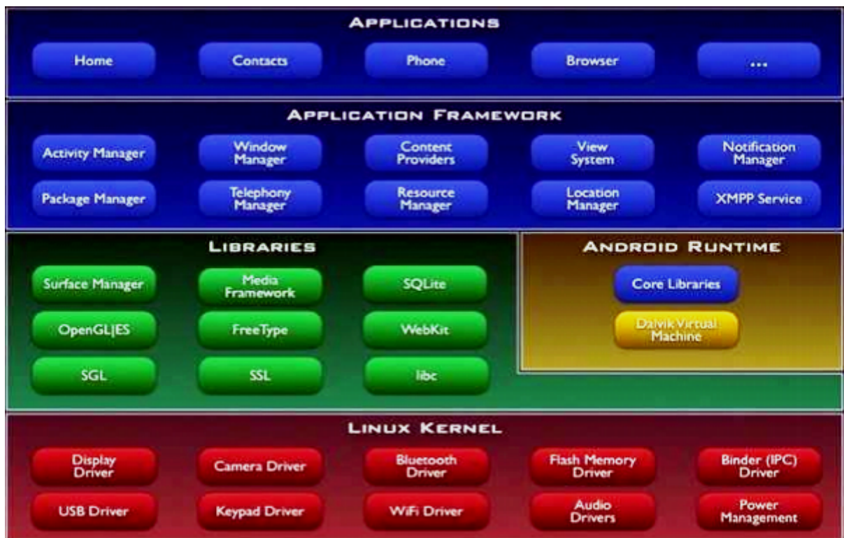
FIGURE 49 – Architecture de la plateforme android
